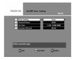
**Channel Name:** You can select channel from the TV or Radio list by pressing **LEFT/RIGHT** button on the remote control.
